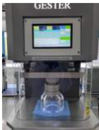
Figure 5a) Burst Resistance in Dry and Wet Conditions Using the Hydraulic Method analyzer
