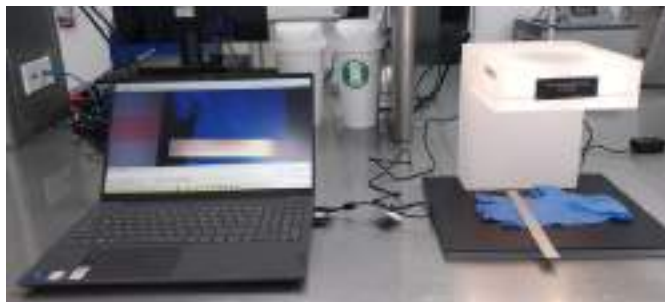
Figure 9a) Automated width tester for gloves
